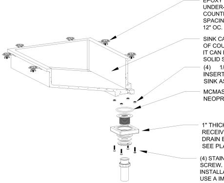
EPOXY SINK CLIPS PROVIDED FOR UNDER-MOUNTING TO STONE & QUARTZ COUNTERTOPS.
