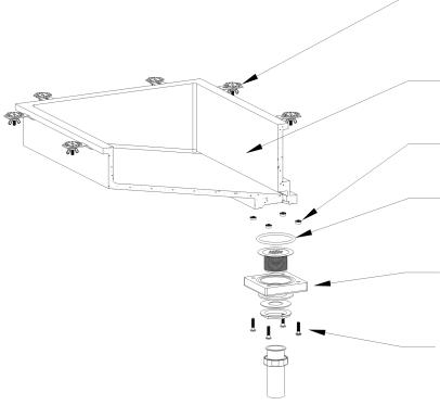
EPOXY SINK CLIPS PROVIDED FOR UNDER-MOUNTING TO STONE & QUARTZ COUNTERTOPS .
